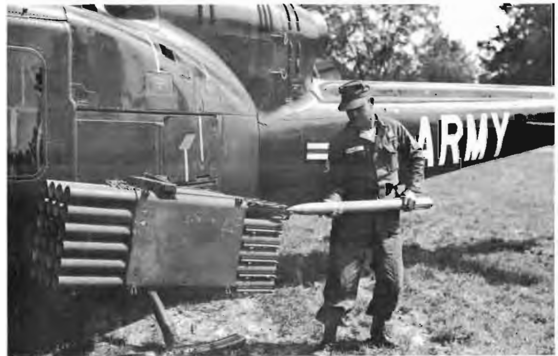
Georgia, 1965. Loading a 2.75 inch rocket into the weapons system mounted on a UH-1B helicopter in preparation for a firing demonstration during test exercise SKY SOLDIER I
