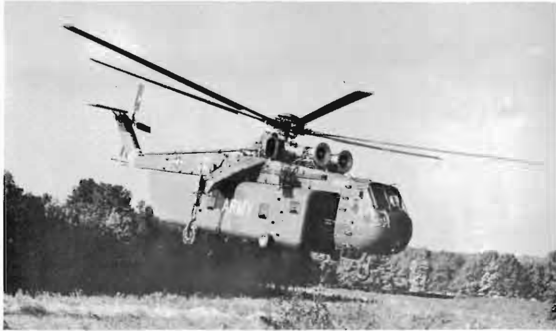
The CA-54A SKYCRANE with pod which can carry 64 troops (at Fort Jackson, South Carolina, November, 1964)
